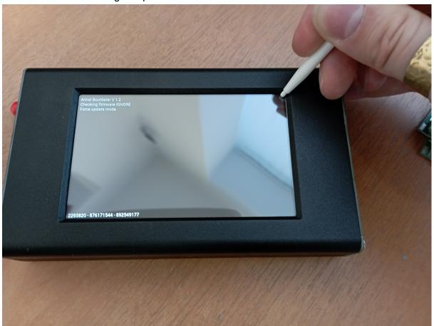
5. Connect the device to the PC via usb cable and proceed to install the firmware as per usual procedure. Note, that your device will report it's firmware version as 0.0.0. This is intentional and should not be considered an issue.
